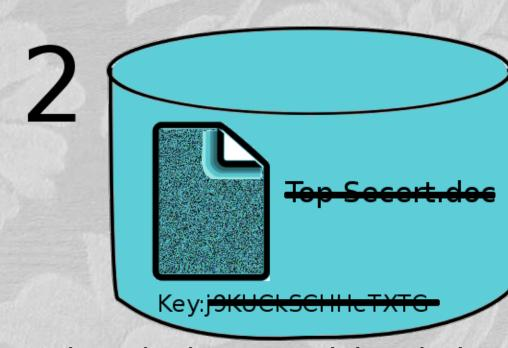
When the key gets deleted, the undelete programs cannot recover the file. That is because the file was encrypted with the deleted key.
