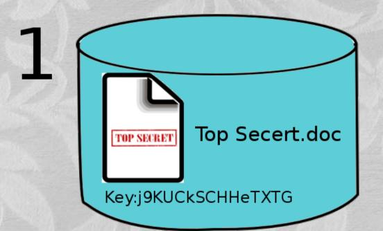
Each file gets encrypted and stored in a database with a diffrent key.
